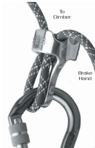
Rigged for belaying with single 9.4mm or larger ropes
